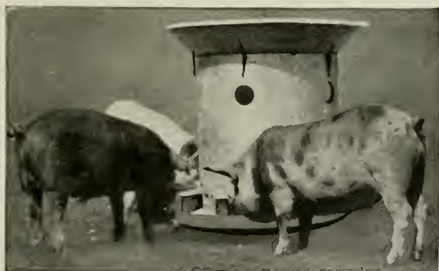
FIG. 47.—Hog motor grinder and feeder. With this machine hogs grind their own feed.
